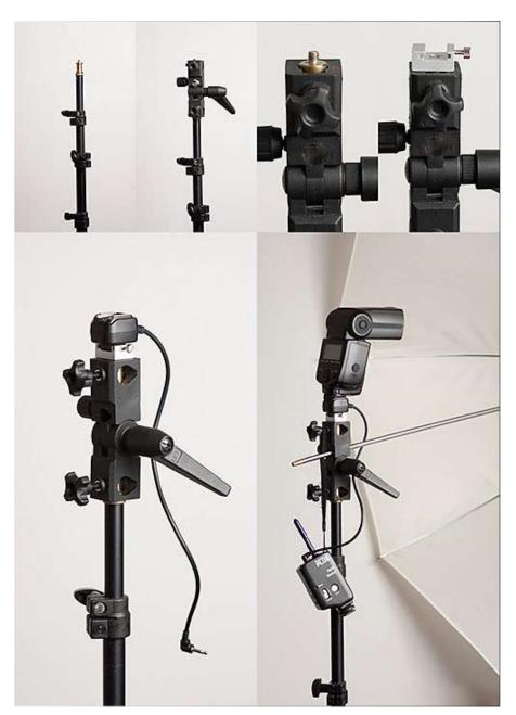
As shown in the picture, make sure the angle adjusting knob/lever of the umbrella adapter is on the RIGHT hand side as the flash is pointed away from you. The angle of the hole that holds the umbrella in place is setup so that it only works properly this way. Your flash will not be angled correctly into the umbrella otherwise.
